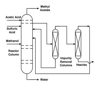
Fewer vessels, pumps, flanges, valves, piping, instruments....
