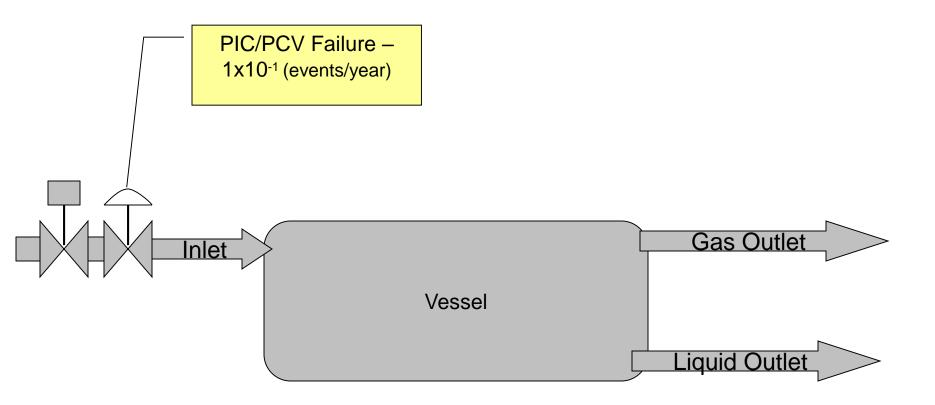
Result – The inherent risk of over pressuring the vessel is the sum of the causes which is  $1.0 \times 10^{-1}$  events/year or 10% chance or an event every 10 years.
