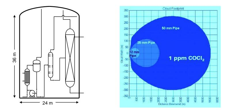
The containment building and small pipe moderates the consequence of a leak, accident or failure.
