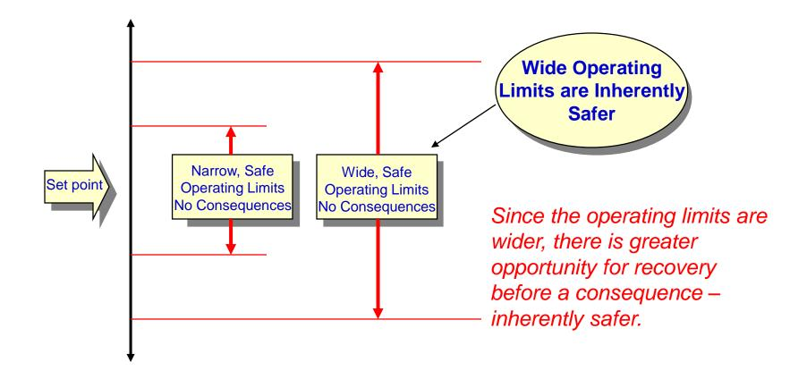
When developing a process design, we have typically worried about the robustness in the design specifications and equipment sizes. We want to incorporate safety concerns into our considerations.
