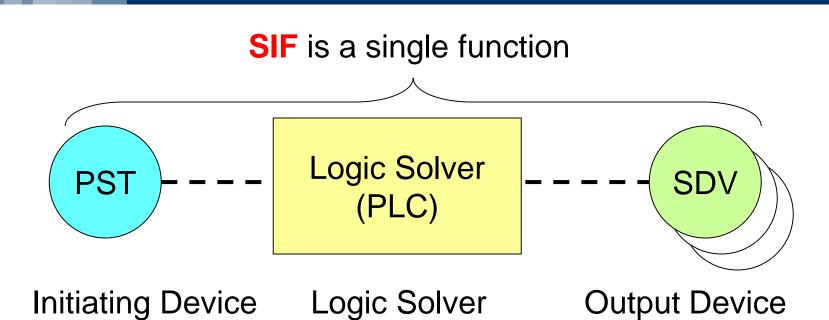
**SIL** is the strength of the SIF, how reliable does it need to be.
